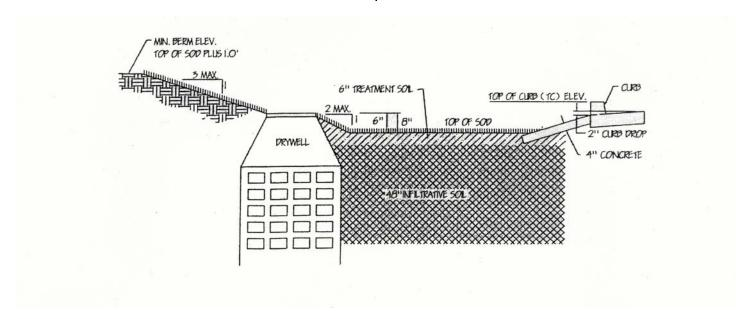
Grassy Drainage Swale - Typical Cross Section
