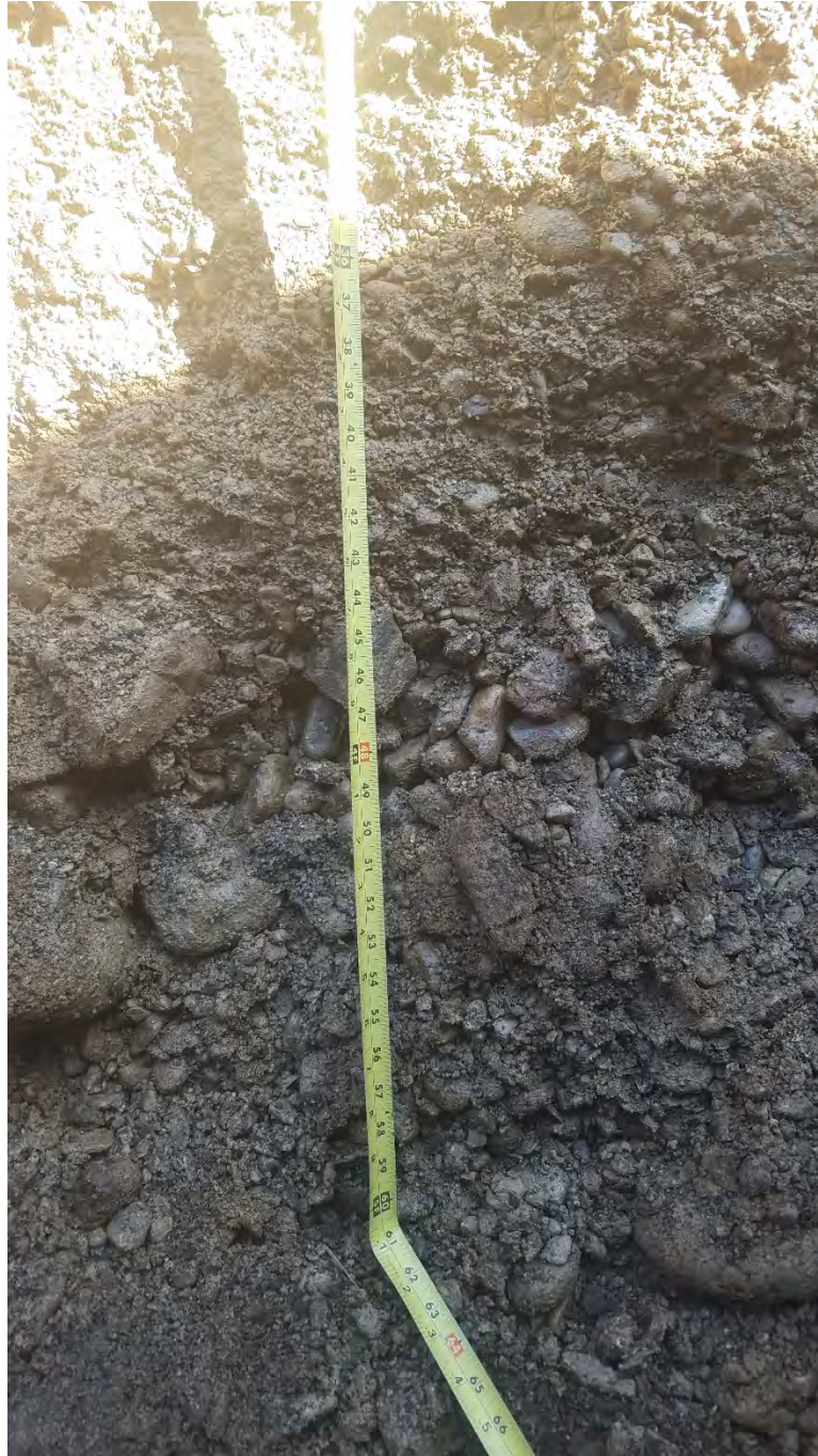
Photograph 4. Bear Creek Site Soil Profile. The photo shows the coarsening with depth and relatively clean gravels below a surface horizon that contained a hardpan layer comprised of iron oxides at 2 feet bgs.
