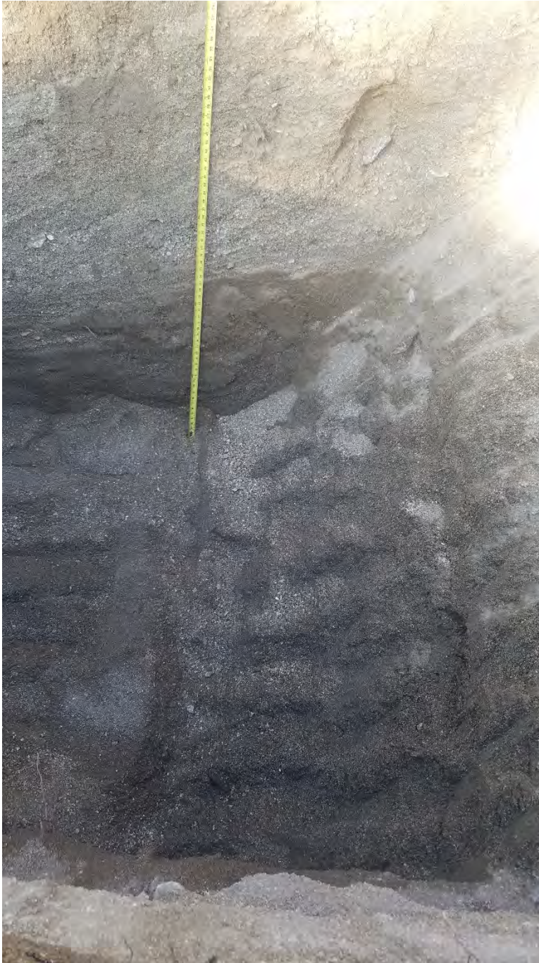
Photograph 3. Dry Creek Site Soil Profile. Photo shows crossbedding in the top portion of photo. Over excavation revealed lateral spreading of the wetting front in the soil profile. The water spread at the contact between forest and bottom set likely due to a change in vertical hydraulic conductivity.
