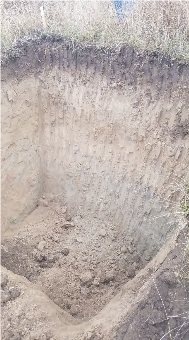
Photograph 2. Deadman Creek Site Soil Profile. Changes in color correspond with change from sandy silt to silt to fat clay with depth.
