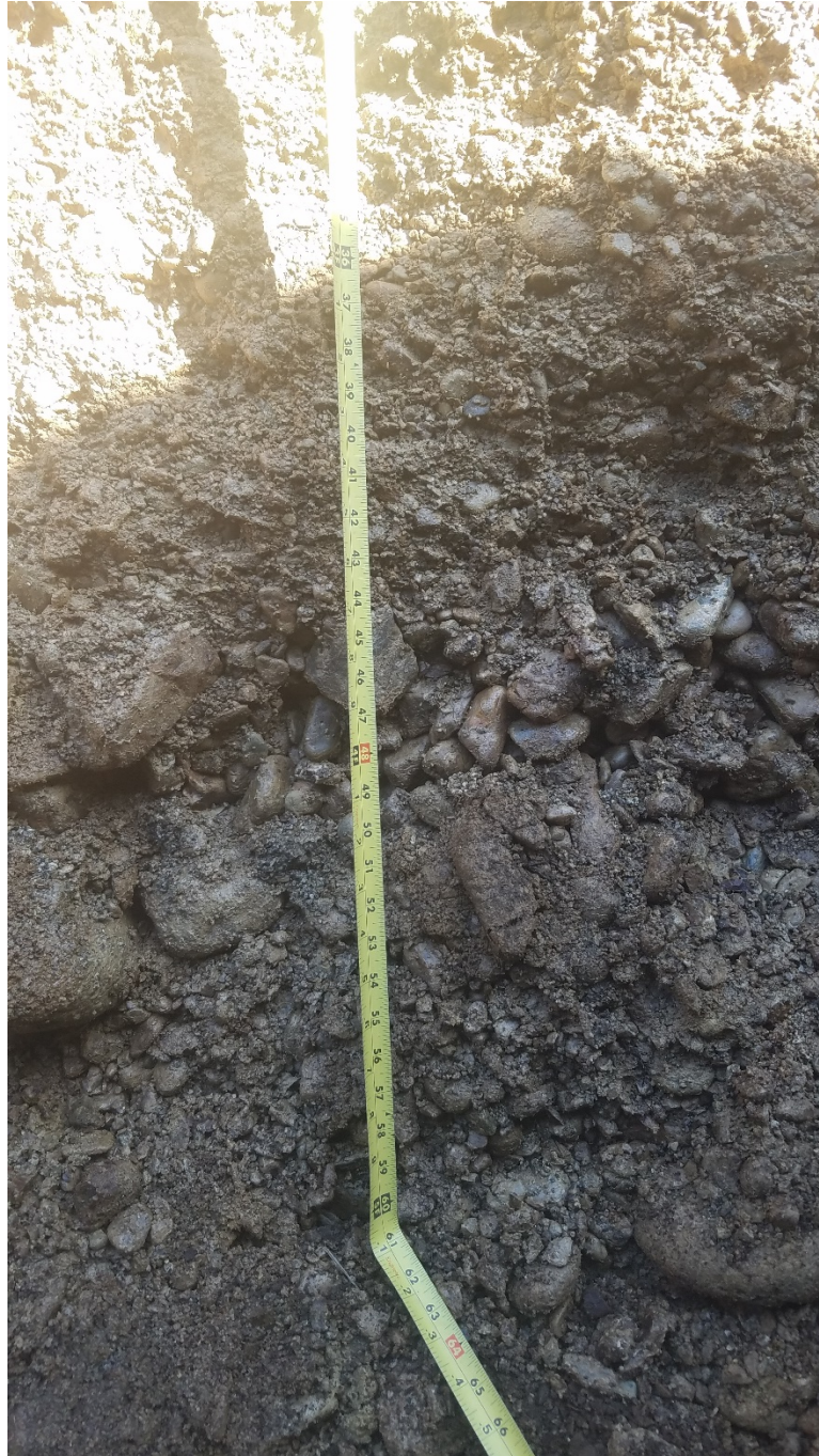
Photograph 4. Bear Creek Site Soil Profile. The photo shows the coarsening with depth and relatively clean gravels below a surface horizon that contained a hardpan layer comprised of iron oxides at 2 feet bgs.
