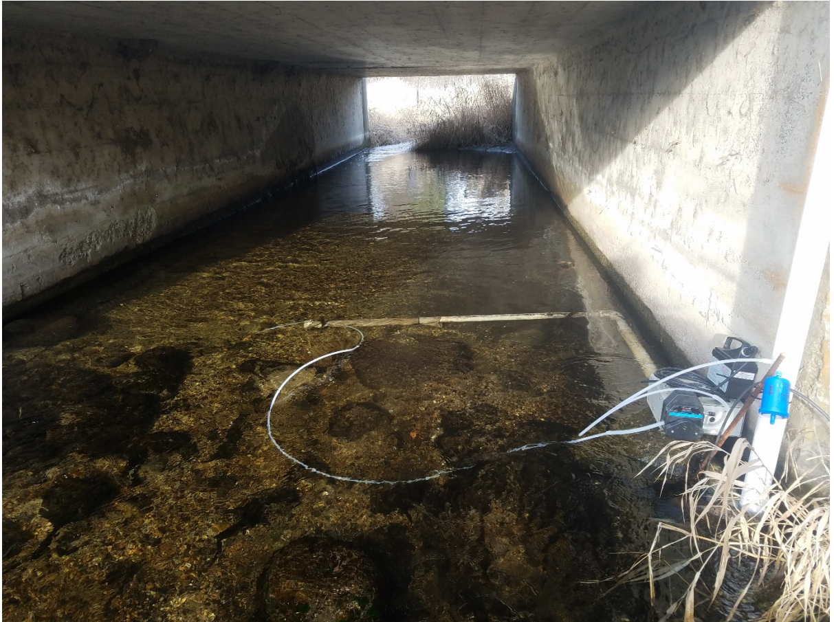
Photograph 1. Bear Creek surface water station. The photograph shows the use of a peristaltic pump to collect total and field filtered water quality samples.
