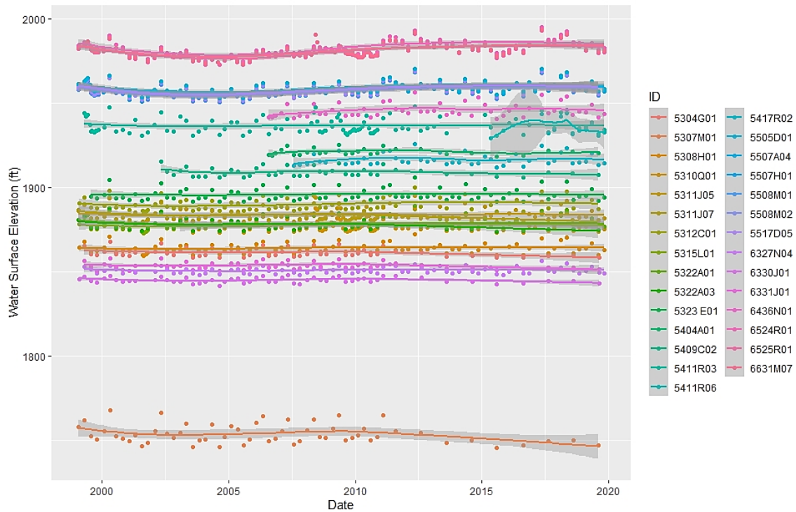
Figure 44. Groundwater surface elevations (WSEs) measured at 28 monitoring wells over the 20-year period between 1999 and 2019.
