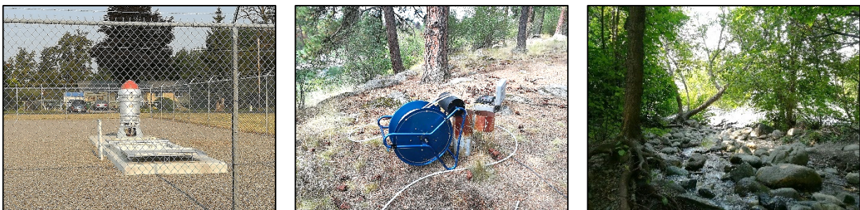
Figure 52. Pictures showing a purveyor well (left), monitoring well (middle), and a natural spring (right). Purveyor wells have infrastructure to pump and convey large volumes of water. Monitoring wells require a portable pump as shown in the photo. Natural springs can be sampled at the surface like a stream.
