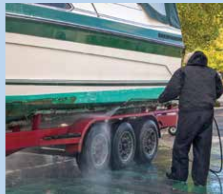
Boat washing wastewater should not discharge to the ground
