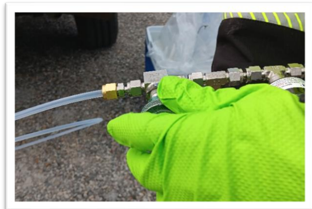
*Figure 11i - Close Effluent when stable
