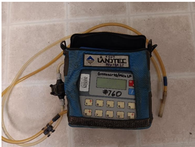
*Figure 4a – GEM(Gas Extraction Monitor) 500 Gas Analyzer
