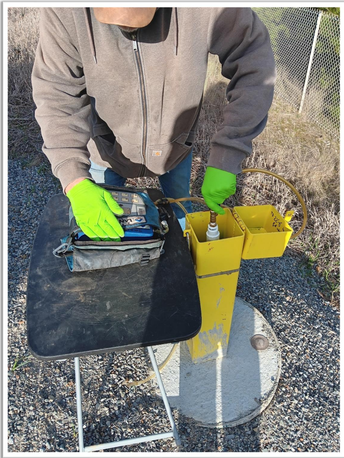
*Figure 8 - Probe Initial Pressure
