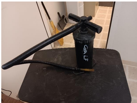
*Figure 4b - Manual Purge Pump
